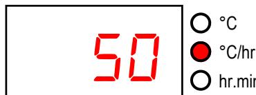
→ then displays ramp rate 1 in the range 1 to 999°C/hr or *FULL* or *End*. This can be altered with the **↑** & **↓** keys. RAMP 1 lamp on the mimic display will flash.
