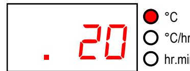
If the left-hand decimal point is on then the keyboard is locked & the ST312A will not respond to the START/STOP key. Press the ↑ & ↓ keys together & hold down for 5 seconds to unlock.
