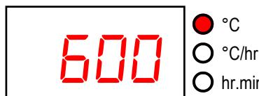
→ then displays temperature t1 in the range 0 to 1320°C. This can be altered with the **↑** & **↓** keys. The t1 lamp on the mimic display will flash.
