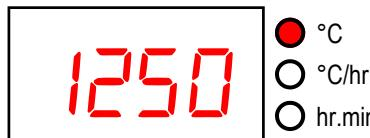
→ then displays the soak temperature in the range 0 to 1320°C. This can be altered with the **↑** & **↓** keys. The SOAK TEMPERATURE lamp on the mimic display will flash.
