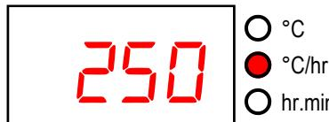
→ then displays ramp rate 2 in the range 1 to 999°C/hr or *FULL* or *End*. This can be altered with the **↑** & **↓** keys. The RAMP 2 lamp on the mimic display will flash.
