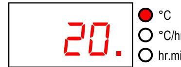
If no delayed start has been set (00.00) then pressing the START/STOP key causes firing to commence immediately. The RAMP 1 lamp on the mimic panel will light. If kiln heating is required then the right-hand decimal point on the display will light while heating power is being applied to the kiln.
