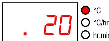
If the left-hand decimal point is on then the keyboard is locked. Press the **↑** & **↓** keys together & hold down for 5 seconds to unlock.
