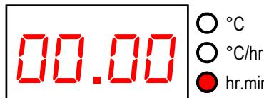
The first push of the **→** key displays the start delay time in the range 00.00 to 99.59 (99 hours 59 mins). This can be altered with the **↑** & **↓** keys. The DELAYED START lamp on the mimic display will flash.
