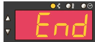
Explanation: the full range of displayed values for ramp rate are: End, 1...999°C/hr, FULL. To mark the end of a program select a ramp rate of "End" by holding down the **DOWN** key until End is displayed. To add an extra segment press the **UP** key until your desired ramp rate is shown. If you want to heat at full power hold down the **UP** key until FULL is displayed.
