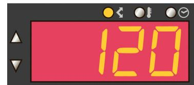
Press the **STEP** key again. The soak temperature in °C is now shown. This can be changed as required with the **UP** or **DOWN** key. Note: the maximum temperature available will be limited by the kiln type. Hold **UP** or **DOWN** key down to get accelerated change of the displayed value.
