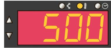
Press the **STEP** key again. The soak time in hours.minutes is now shown. This can be changed as required with the **UP** or **DOWN** key in the range 00.00 (no soak) up to nearly 100 hours. Note: hold **UP** or **DOWN** key down to get accelerated change of the displayed value.
