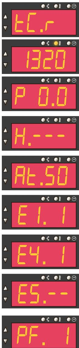
The currently configured thermocouple type letter will flash. This can be altered with the ▲ & ▼ keys to R,S,K or N type (-SHN). Press the ►■ key.
