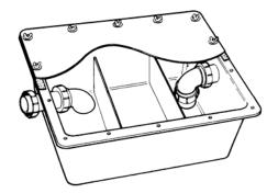
The Clay Trap measures  $552 \times 400 \times 270$ mm deep and has a 20 litre capacity. The cut-away lid, in our illustration reveals the two weirs, the inlet on the left and the outlet, which has a 76mm water seal on the right. Both inlet and outlet have coupling nuts for joining to 38mm 'Vulcathene Mechanical' pipe. The lid, which has a sealing ring, is retained in position with fourteen wing nuts.
