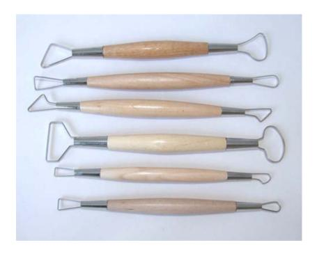
A set of 8" and 6" ground edge tools that are ideal for carving into soft and leather clay when modelling or equally useful for turning the bottom of thrown pots.
