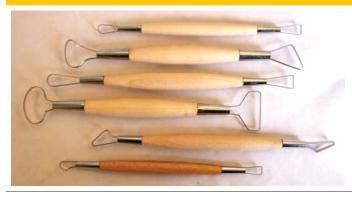
A selection of six double ended Ground Edge Tools with hardwood handles. Stainless steel blades with ground cutting edge. Ideal for turning on the wheel and carving and slicing when modelling.
