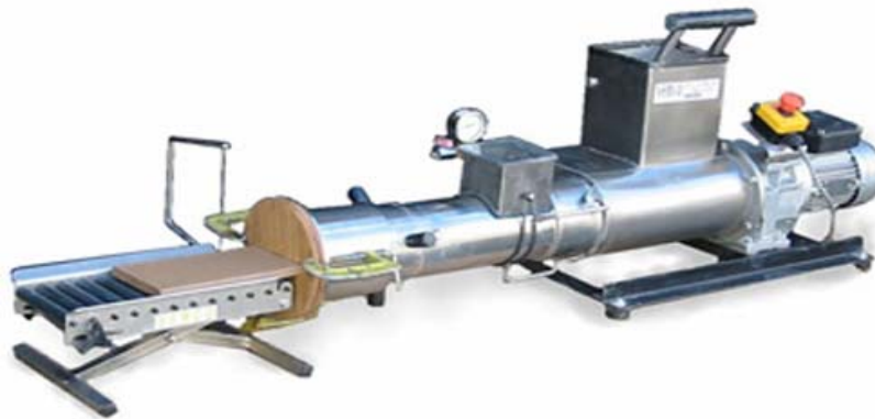
Super-twin shown making 125mm (5") tiles with the expansion chamber module
